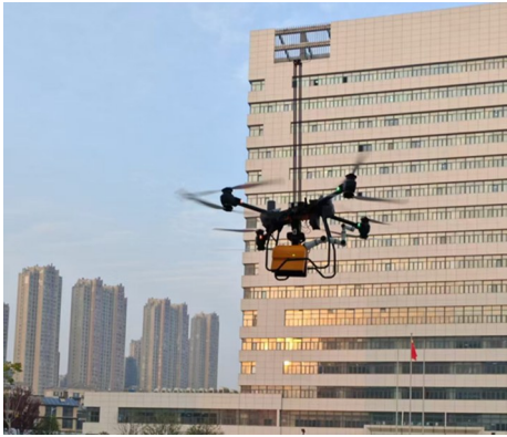
图8 飞行机械臂施工作业场景图 Fig.8 Scenario diagram of flying manipulator operation
