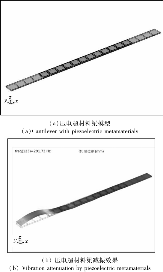
图5 压电超材料梁及减振效果 Fig. 5 Piezoelectric metamaterial beam and attenuation effect
